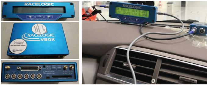
Fig. 10. Telematics BOX records the ground truth for the rotation angle of steering wheel.
